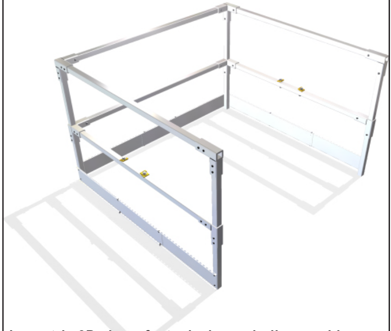
Isometric 3D view of a typical guardrail assembly
